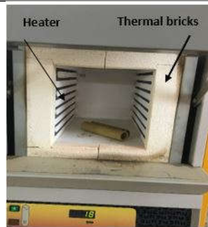
Fig. 4 Kiln furnace used for firing pottery tubes.
