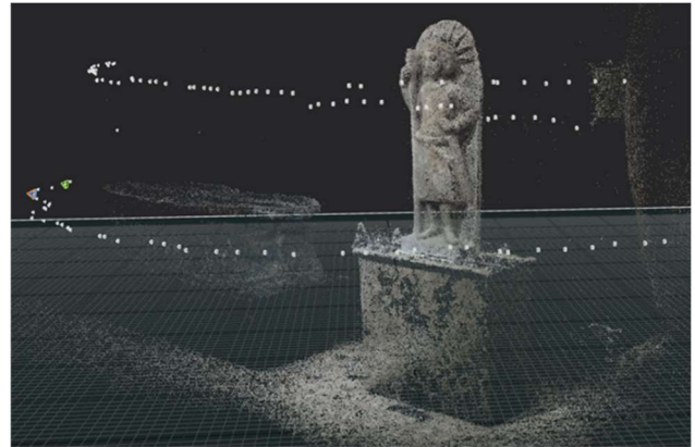
Figure 5: Image acquisition scenario, as it is required by SfM photogrammetry with large overlaps and different locations and angles [13].
