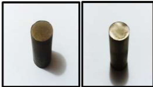
(a) Before grinding and polishing (b) After grinding and polishing
