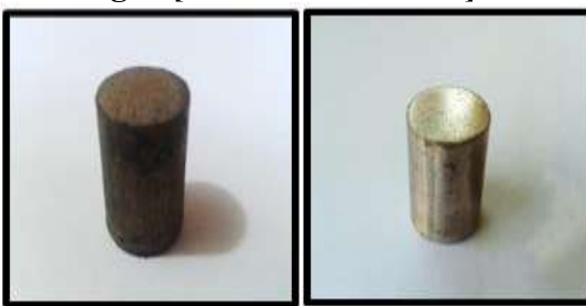
(a) Before grinding and polishing (b) After grinding and polishing
