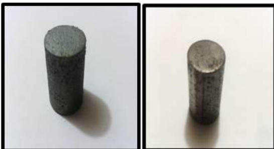
(a) Before grinding and polishing (b) After grinding and polishing
