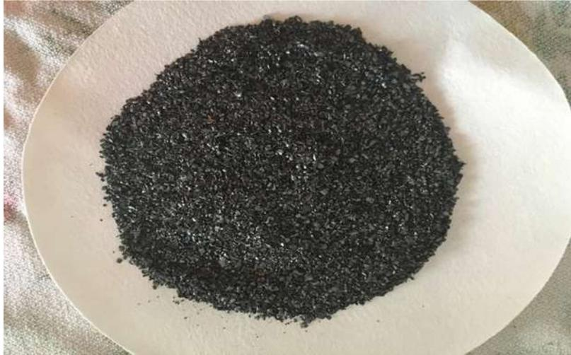
**Fig.1: Prepared ZVI from scrap iron.**
