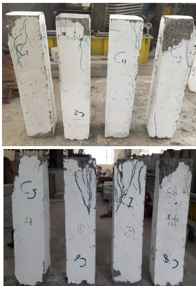
Fig.5 Crack Patterns of Tested Columns (Solid and Hollow section).
