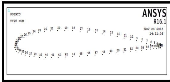
Fig. 1 Outlines of NACA 0015 airfoil
