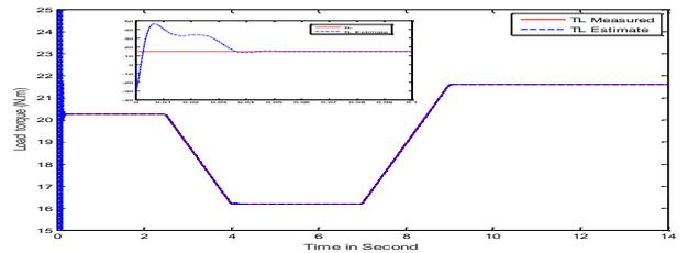
**Fig.6. Measured and estimated load torque variation measured in (N. m)**
