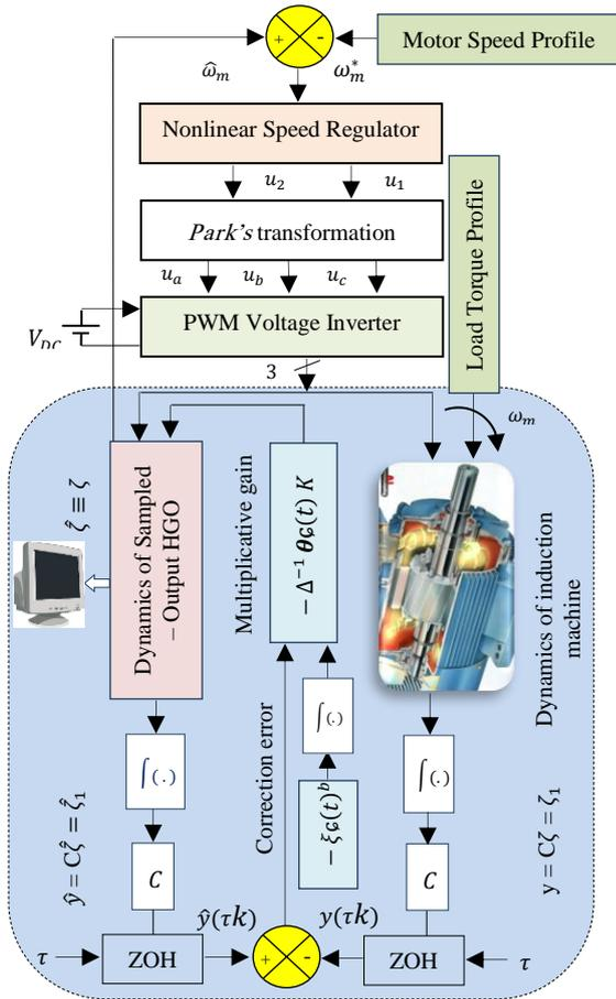
**Fig.1. Induction motor drive running with high gain state observer**
