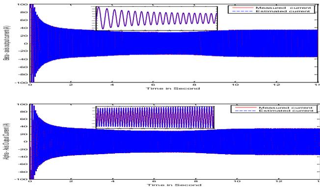
**Fig.2. Measured, and estimated (α - β) currents measured in (A)**
