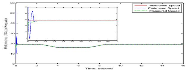
**Fig.5. Reference, measured and estimated rotor speed measured in (rad/sec)**
