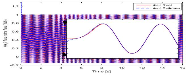
**Fig.3. Measured and estimated (α - β) rotor flux measured in (Wb)**
