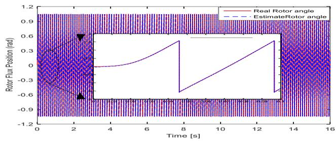
**Fig.4. Estimated and real rotor flux position measured in (rad)**
