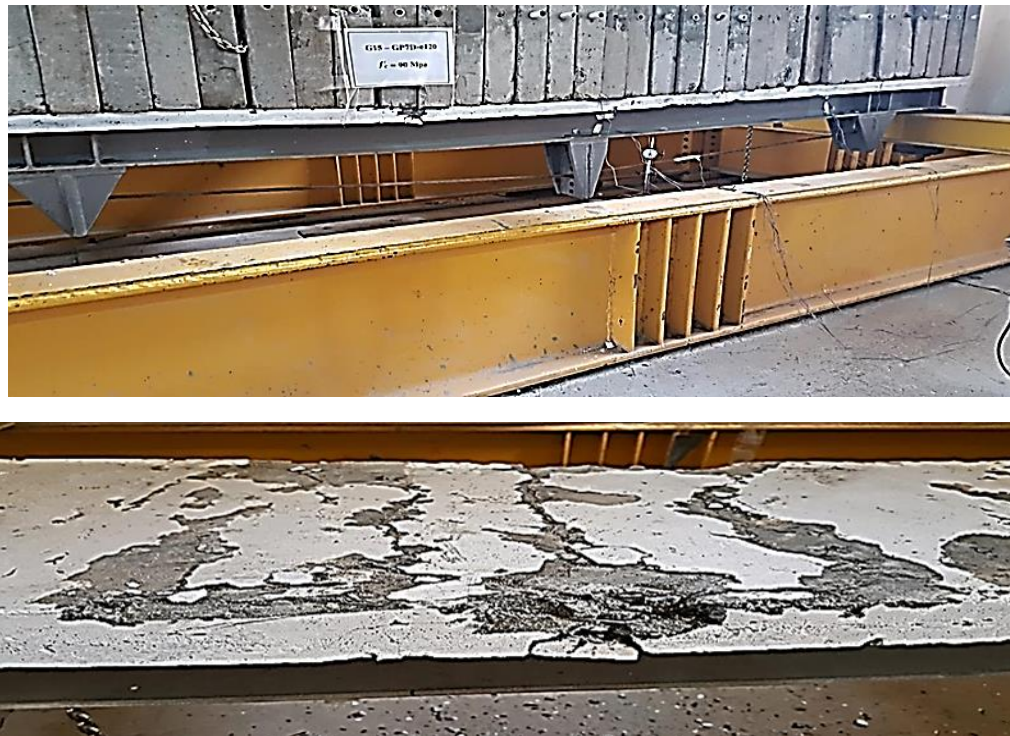
Fig. 18 The Mode of Failure of the Steel Girder (GP7D-e200) G5
