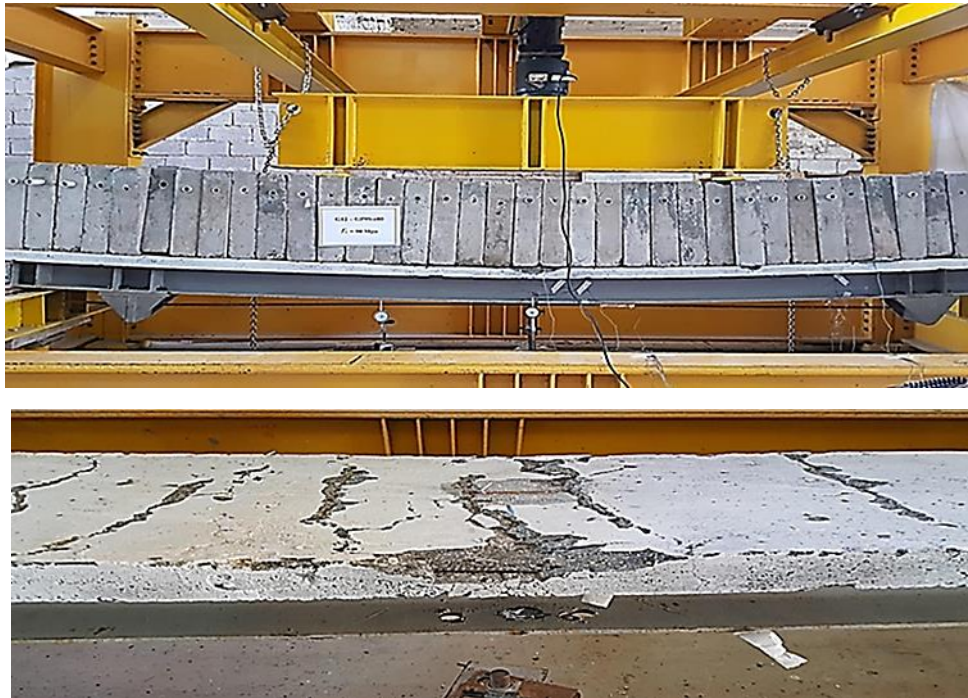
Fig. 13 The Mode of Failure of the Steel Girder (GP9S-e80) G2
