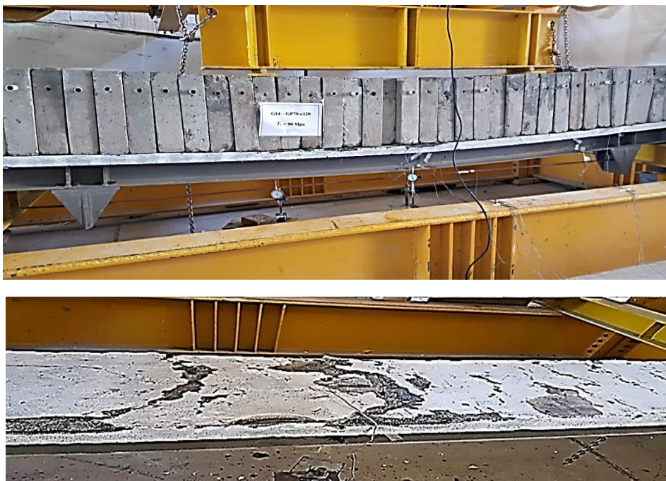
Fig. 17 The Mode of Failure of the Steel Girder (GP7S-e120) G4
