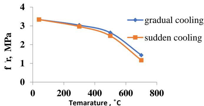
Fig. 4 Burning temperature versus modulus of rupture.
