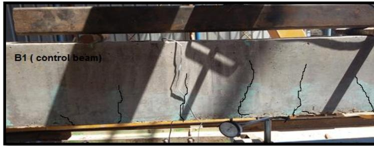
**Plate 4. Failure mode of reference beam R.**
