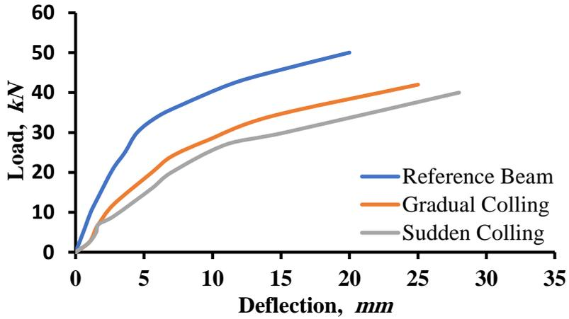
Fig. 12 Load- midspan deflection of group I beams which burned at 300 °C and R beam.
