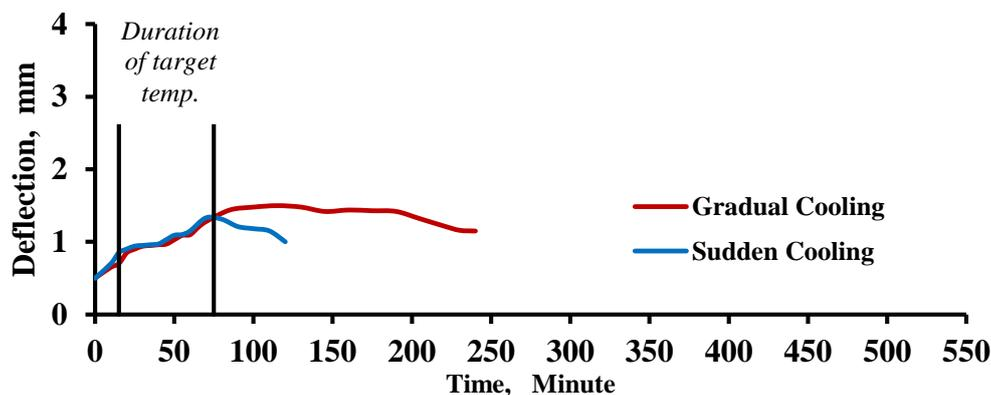
Fig. 5 Midspan camber -time history for group I beams which burned at 300 °C.
