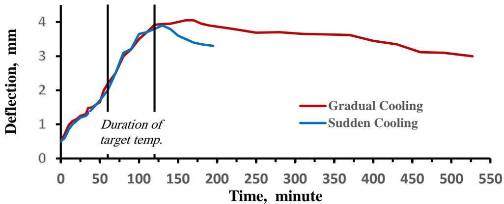
**Fig. 7** Midspan camber -time history for group III beams which burned at 700 °C.
