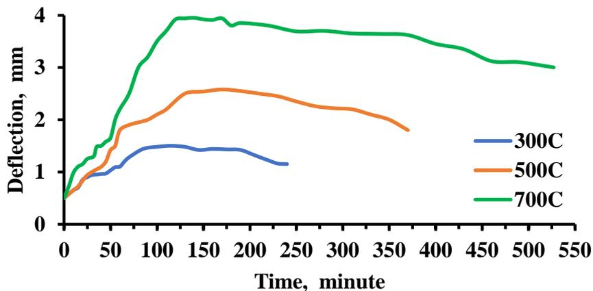
Fig. 9 Midspan camber -time history for gradually cooled beams G<sub>1</sub>, G<sub>2</sub> and G<sub>3</sub> at different burning temperatures.
