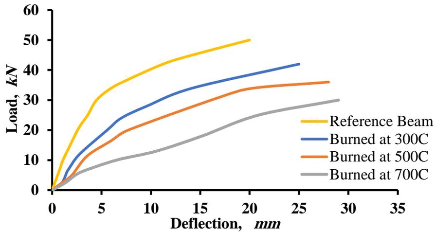
**Fig. 10 Load-midspan deflection for burned beams G<sub>1</sub>, G<sub>2</sub> and G<sub>3</sub> then gradually cooled and R beam.**
