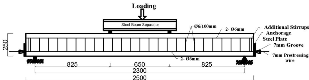
**A- Beam dimensions.**
