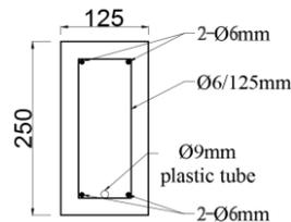
**B- Beam cross section.****Fig. 1 Details of the beam reinforcement.**
