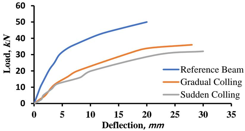
Fig. 13 Load- midspan deflection of group II beams which burned at 500 °C and R beam.
