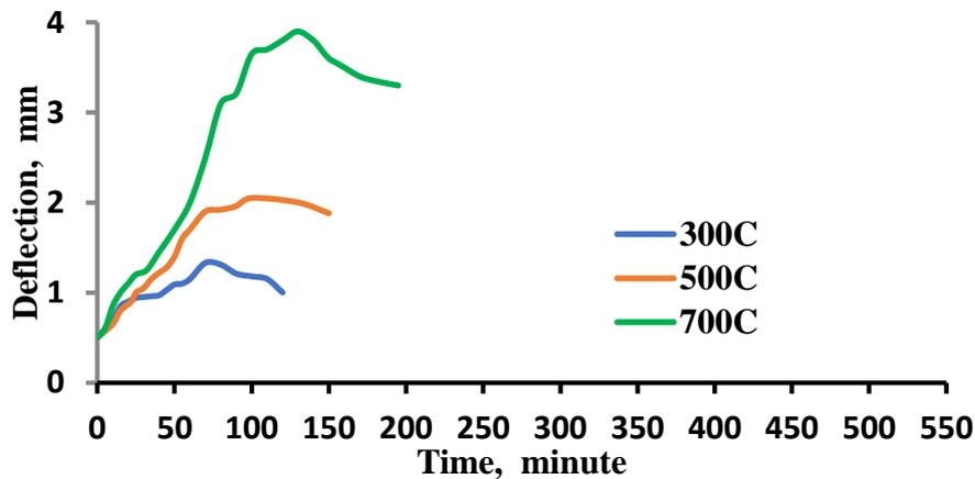
Fig. 8 Midspan camber -time history for suddenly cooled beams S<sub>1</sub>, S<sub>2</sub> and S<sub>3</sub> at different burning temperatures.
