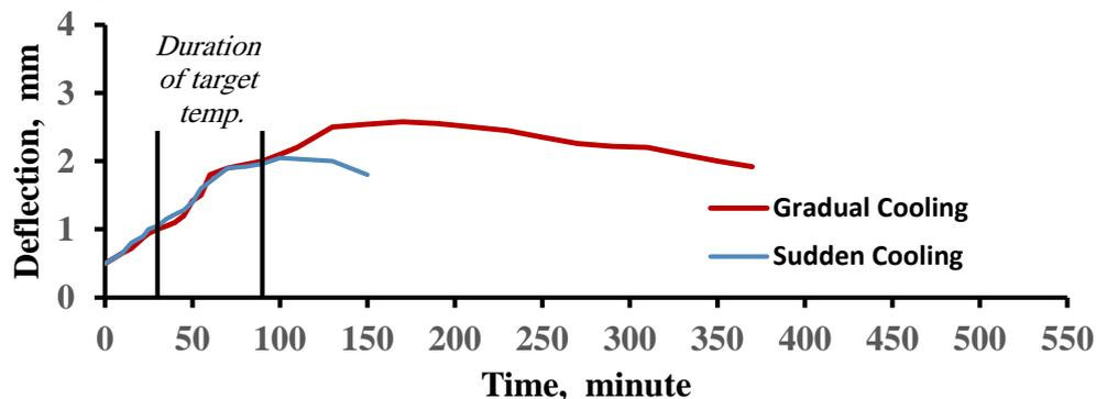
Fig. 6 Midspan camber -time history for group II beams which burned at 500 °C.
