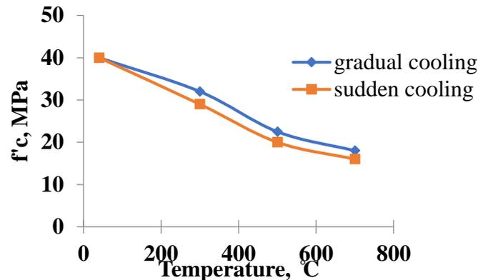
Fig. 3. Burning temperature versus concrete compressive strength.
