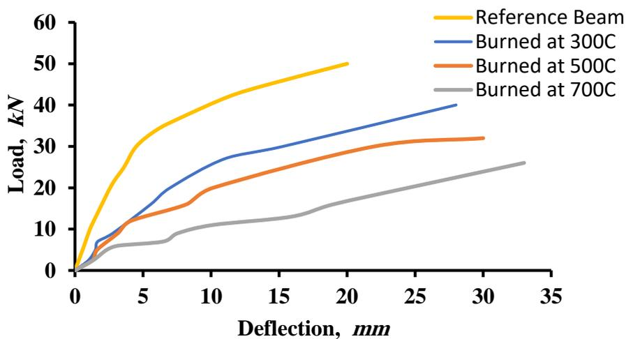
**Fig. 11 Load-midspan deflection for burned beams S<sub>1</sub>, S<sub>2</sub> and S<sub>3</sub> then suddenly cooled and R beam.**
