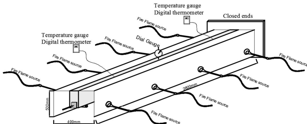
**Fig. 2 Manufactured furnace with the nozzles and other measurements instrumentations during the burning.**
