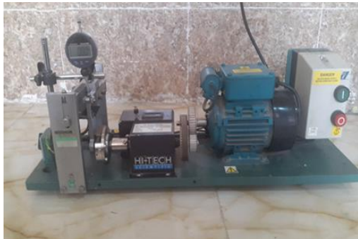
Fig.7 Alternating bending Fatigue Machine
