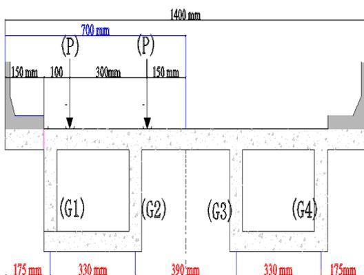
**Fig. 4 Load case (I, II,IV) in the transverse direction (model)**
