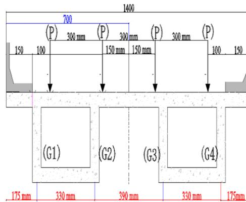
**Fig. 7 Load case (III) in the transverse direction (model)**
