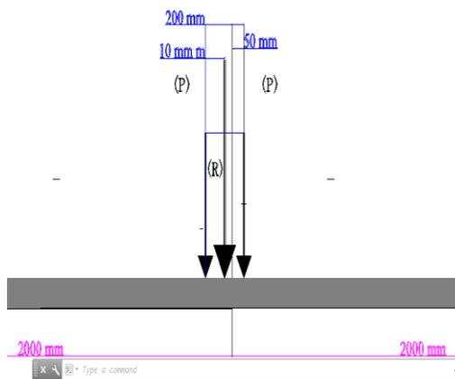
**Fig. 6 Section at mid span; Long direction for load case (IV); axle location of scaled design tandem**
