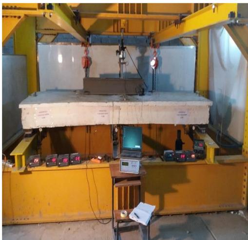
**Fig.12 Design truck at the exterior lane load case (I) for model BGC**
