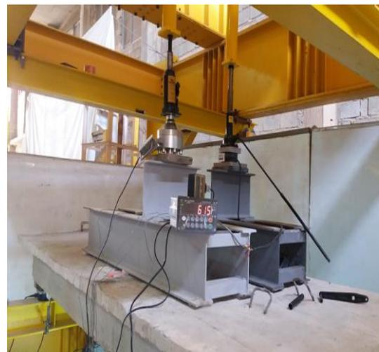
**Fig.14 Load case (III) in the transverse direction (model) BGS**
