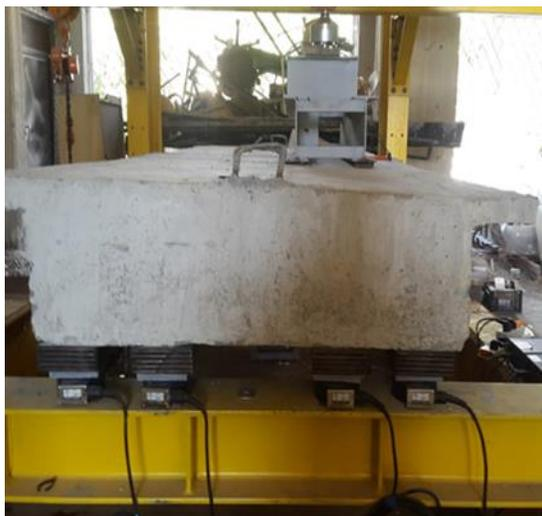
**Fig.8 Load cell under bridge girder**
