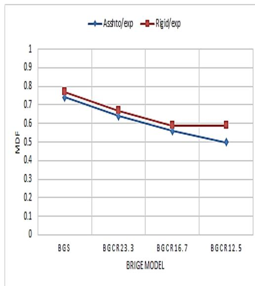
**Fig.17 MDF comparison for the exterior girder under load case III**
