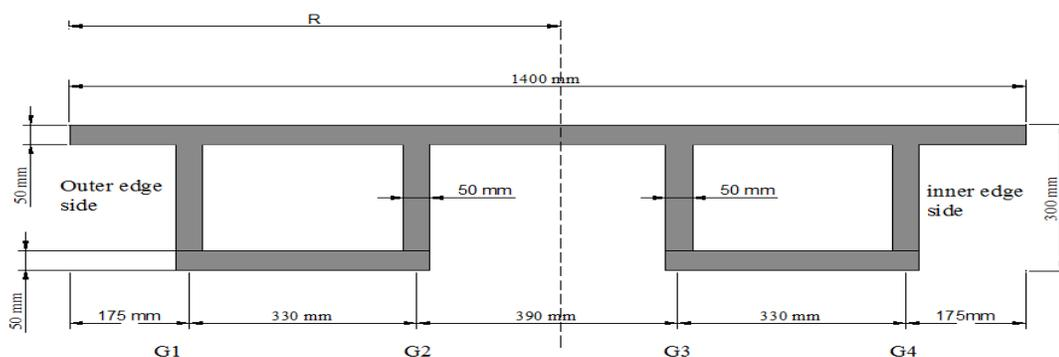
**Fig. 1 Bridge models cross section**
