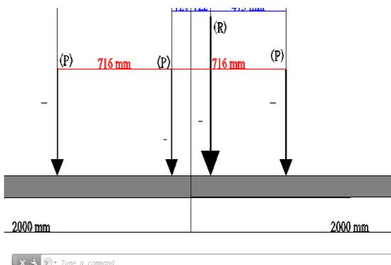
**Fig. 5 section at mid span; Long direction for load case (I, II,III); axle location of scaled design truck**
