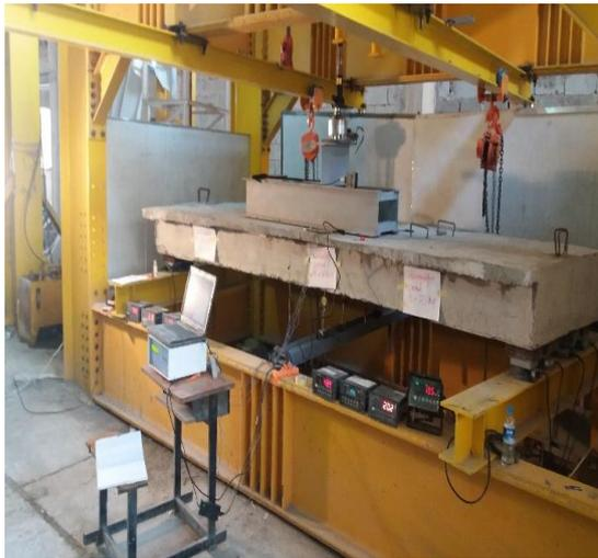
**Fig. 13 Design truck at the internal lane load case (II) for model BGC R12.5**
