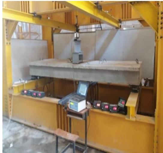
**Fig.15 Design tandem at the external lane load case (IV) for model BGS**
