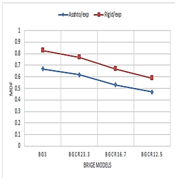
**Fig.16 MDF comparison for the exterior girder under load case I**
