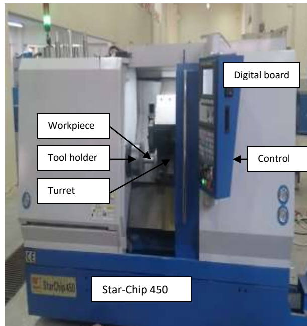
Fig. 1 CNC lathe use in experimental work.
