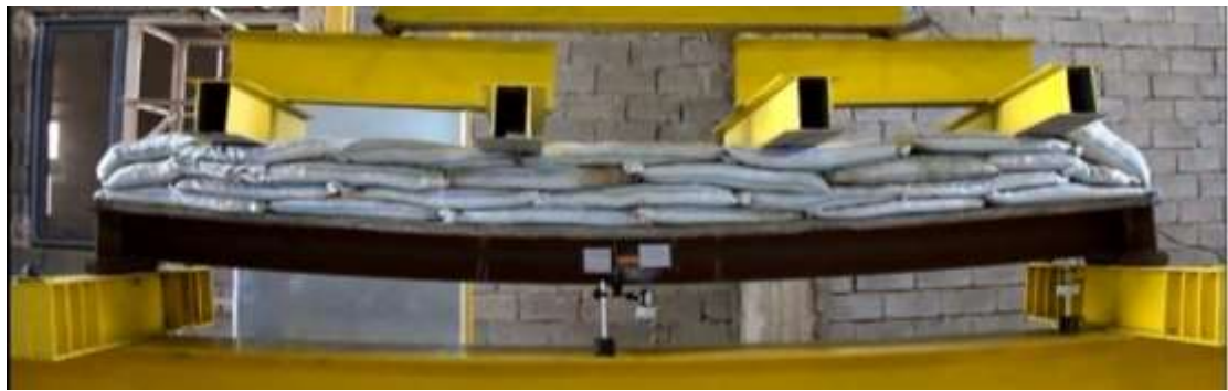
(a) Excessive deflection of SB-RC R just before failure
