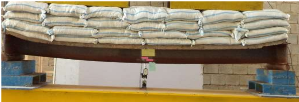
(a) Excessive deflection of SB-RC 700 just before failure
