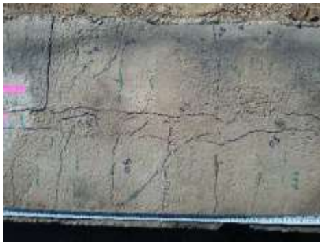
(a) Excessive deflection of SB-RC 500 just before failure
