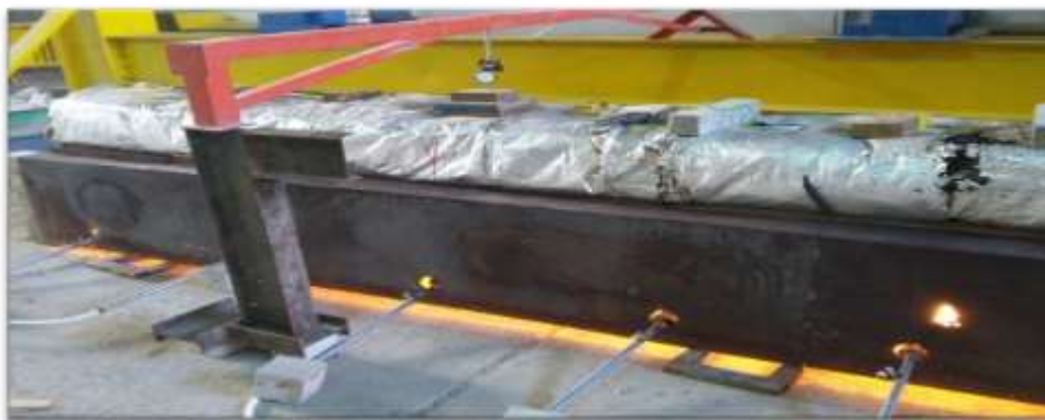
Plate 1 Burning process with applying uniformly distributed load
