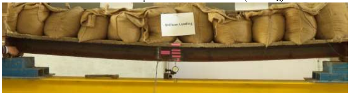
(a) Excessive deflection of SB-RC 300 just before failure
