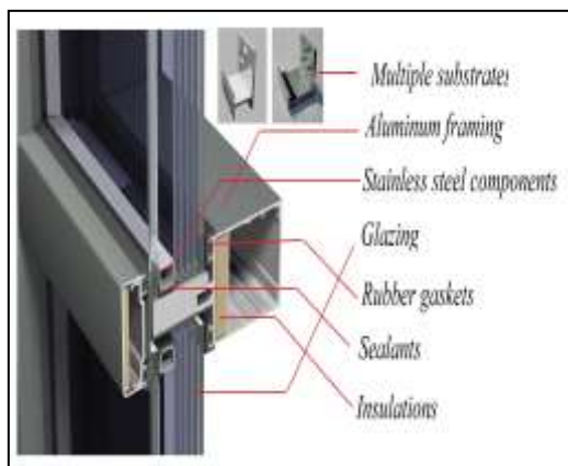
Fig. 2. Example of curtain walls
