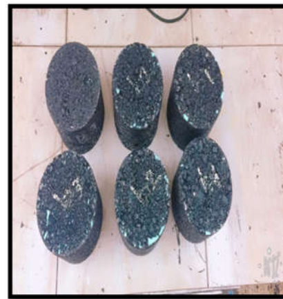
Plate.2 Superpave Gyratory Compactor Samples preparation
