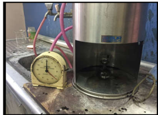
Plate.1: illustrated the physical test for emulsion (Penetration and Saybolt Furol viscosity)
