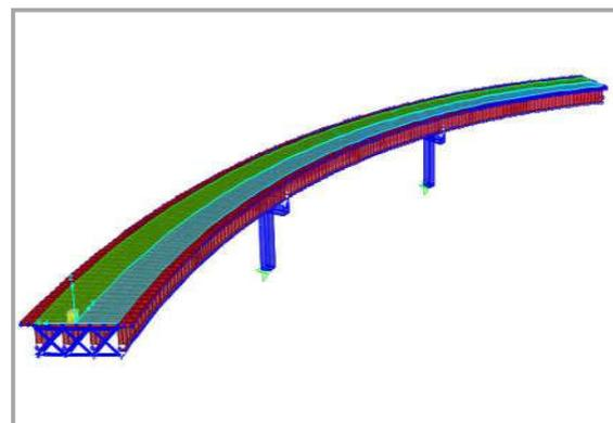
**Fig. 2:** 3D finite element model for the 4-girders curved bridge, cross frames and lanes width are shown.
