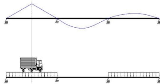
**Fig. 8: Location of the lane load and truck for maximum positive moment in span [5].**
