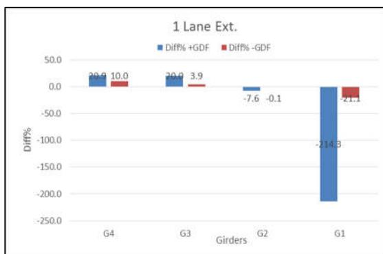
**Fig.18: Percentage difference in GDF values due to curvature change (L/R=0.5) to (L/R=2.4) for exterior lane loading.**
