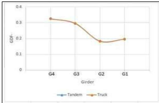
**Fig.7: Negative GDF values due to different types of ASSHTO vehicular live load.**
