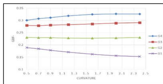
**Fig.14: Effect of bridge curvature on (GDF-) values due to exterior lane load.**
