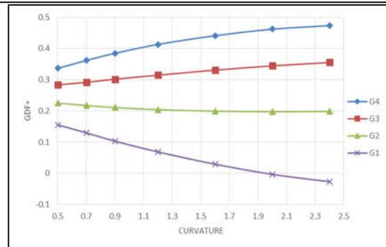
**Fig.11: Effect of bridge curvature on (GDF+) values due to 2 lane loading.**
