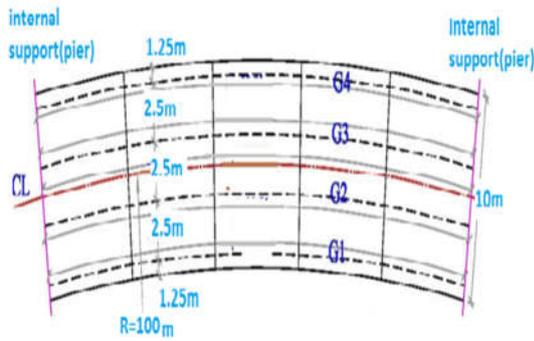
**Fig. 3: Plan of the central span of typical curved bridge with 10m deck width.**
