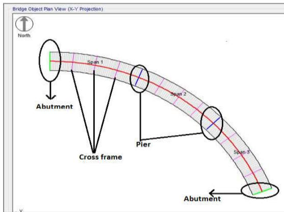
**Fig. 4: CSI-bridge Plan view of the bridge object**
