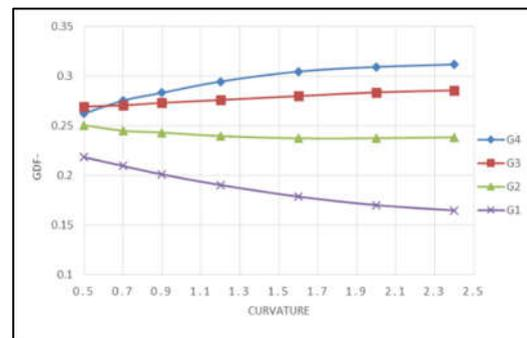
**Fig.12: Effect of bridge curvature on (GDF-) values due to 2 lane loading.**
