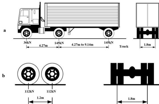
**Fig.5: AASHTO LRFD vehicular loading, (a) truck, (b) tandem [5]**
