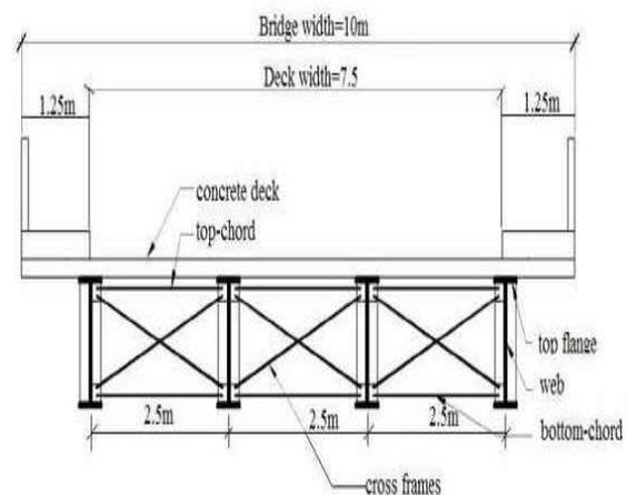
**Fig.1: Typical cross-section of the composite concrete-steel bridge**
