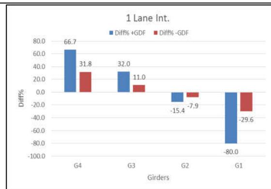
**Fig.19: Percentage difference in GDF values due to curvature change (L/R=0.5) to (L/R=2.4) for interior lane loading**
