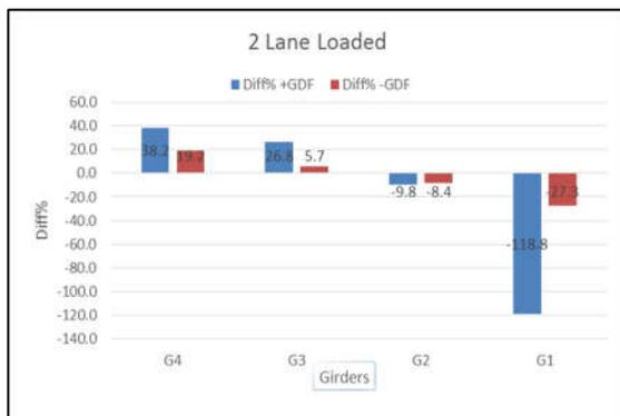
**Fig.17: Percentage difference in GDF values due to curvature change (L/R=0.5) to (L/R=2.4) for 2 lane loading**
