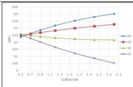
**Fig.15: Effect of bridge curvature on (GDF+) values due to interior lane load.**
