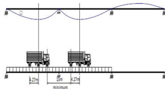
**Fig. 9: location of the lane load and truck for maximum negative moment in span [5].**
