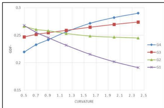
**Fig.16: Effect of bridge curvature on (GDF-) values due to interior lane load.**
