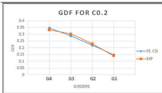
**Fig. 10: Comparison with experimental work for different bridge curvature.**
