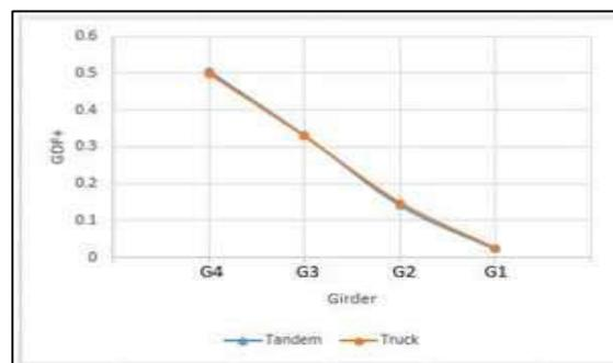
**Fig.6: Positive GDF values due to different types of AASHTO vehicular live load.**
