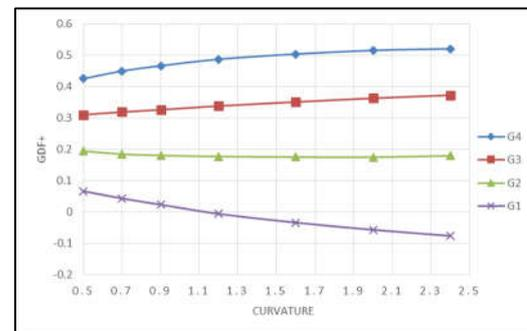
**Fig.13: Effect of bridge curvature on (GDF+) values due to exterior lane load.**
