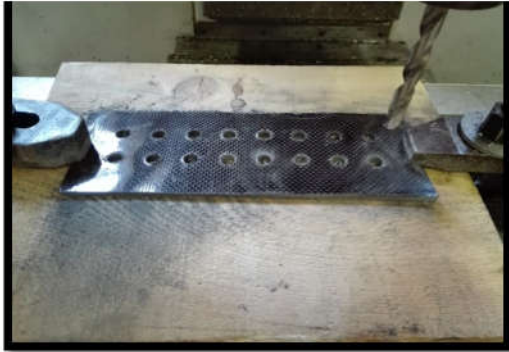
Fig.3 CFRP composite after drilling process.
