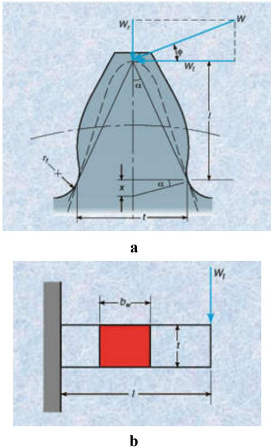
Fig.2 Gear Tooth as Cantilever Beam [8]
