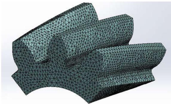
**Fig.5** Three Dimensional model with Mesh for standard Helical gear of helix angle  $22.5^\circ$
