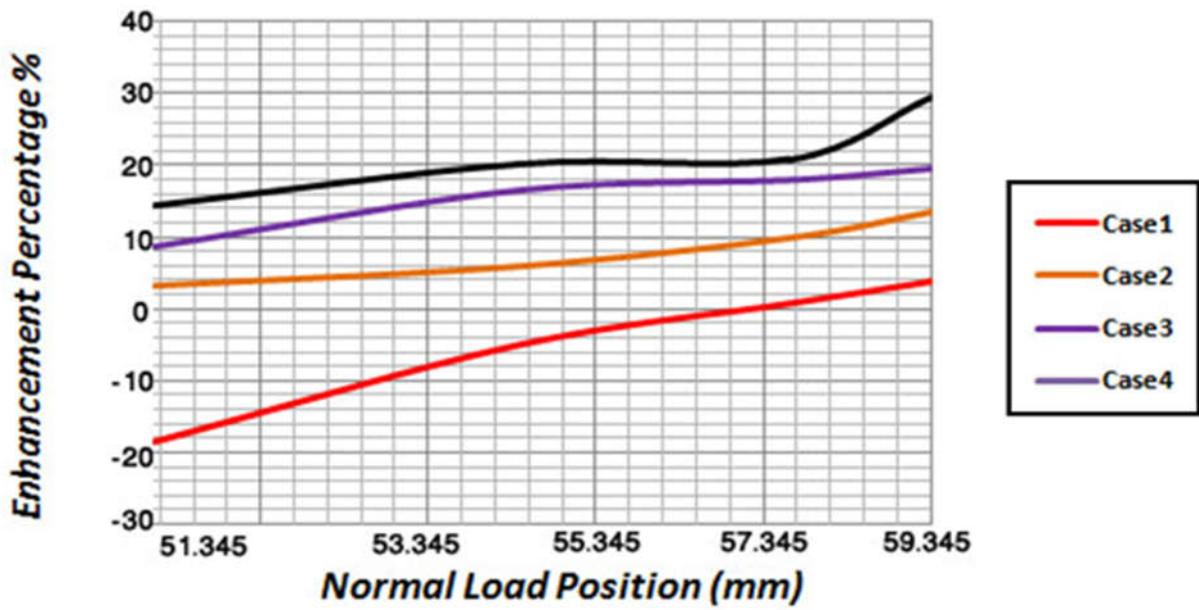
Fig.8 The maximum bending stress at the tensile root fillet when the normal load position varies along the gear tooth profile from tip to root.
