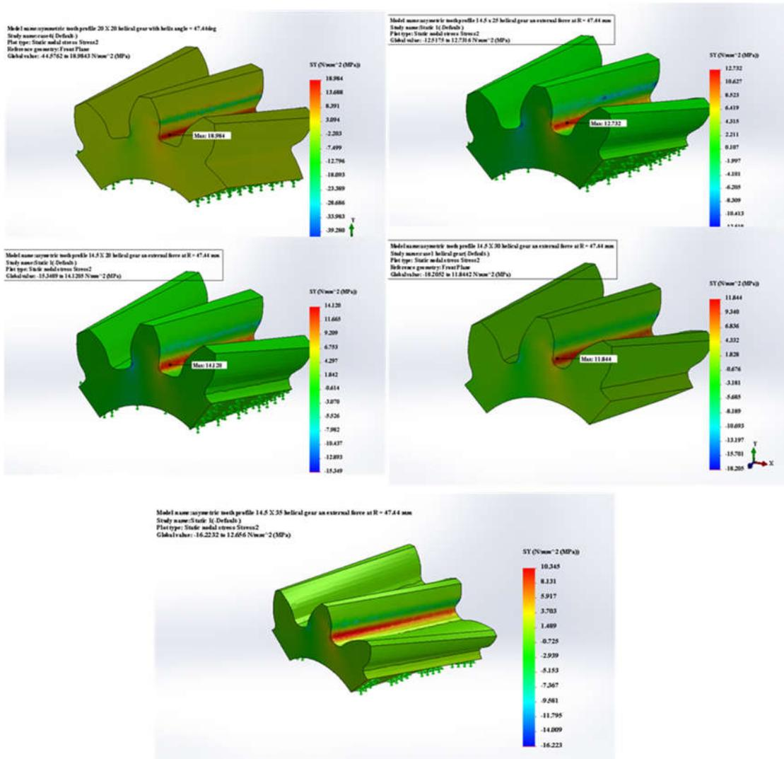
**Fig.7 Three Dimensional bending stress distribution inside tooth of helical gears when the load acts at the root point**
