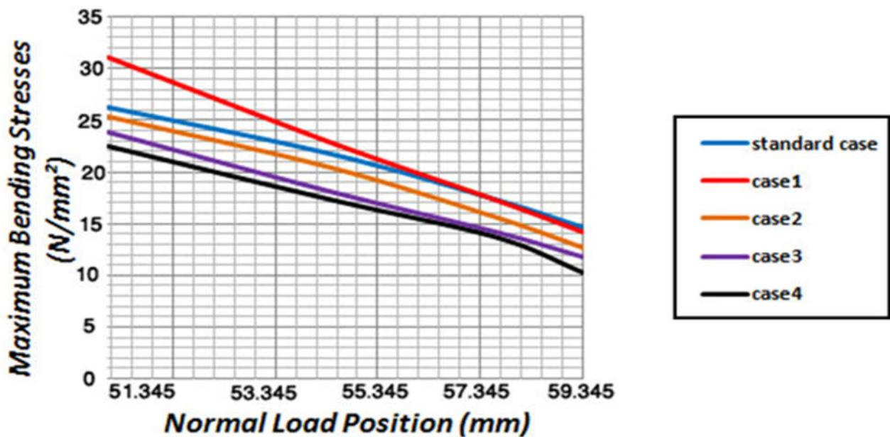
Fig.9 The relationship between the enhancement percentage relative to the standard case with normal load position. When the normal load position varies along the gear tooth profile from tip to root
