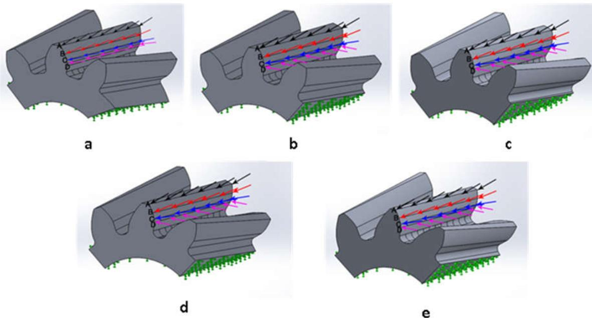
**Fig.4** External normal force is applied with an angle at four position along involute tooth profile for five models. (a) standard helical gear (20/20). (b) asymmetric tooth profile (20/14.5). (c) asymmetric tooth profile (25/14.5). (d) asymmetric tooth profile (30/14.5). (e) asymmetric tooth profile (35/14.5). with boundary condition.
