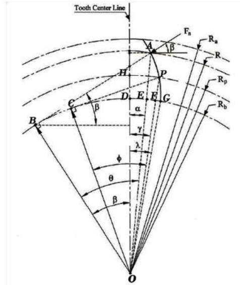
Fig.3 Determination of the loading angle  $\beta$
