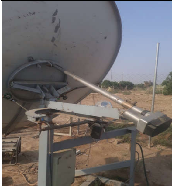
Fig. 3 Tracking system actuators
