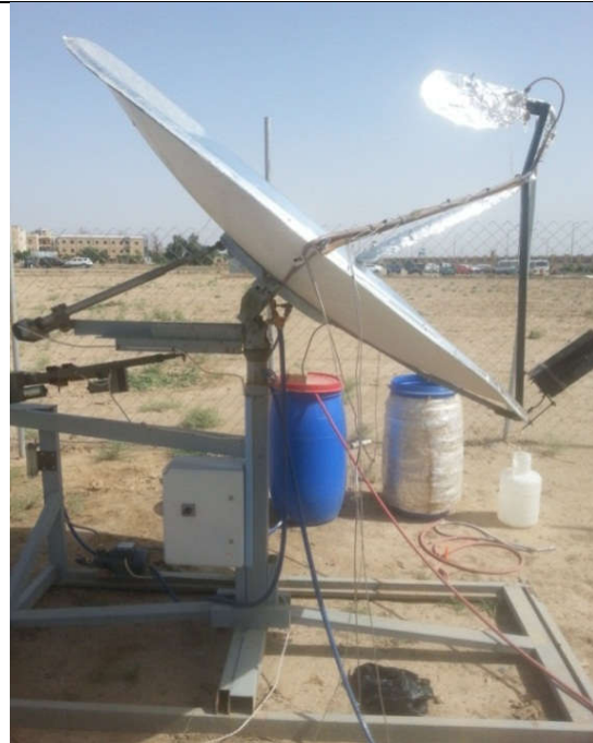
Fig. 1 The used dish solar collector
