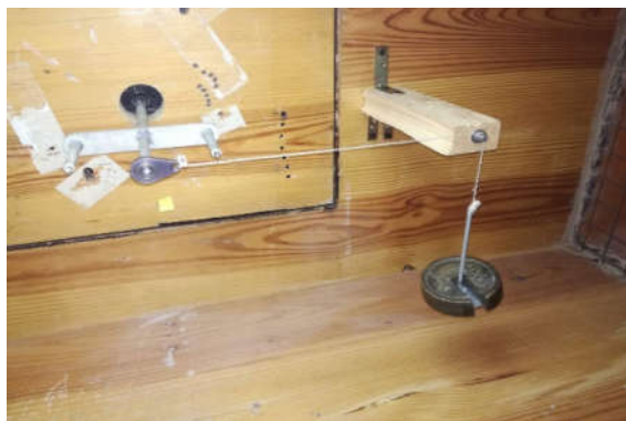
Fig.13 Calibration of drag Spring
