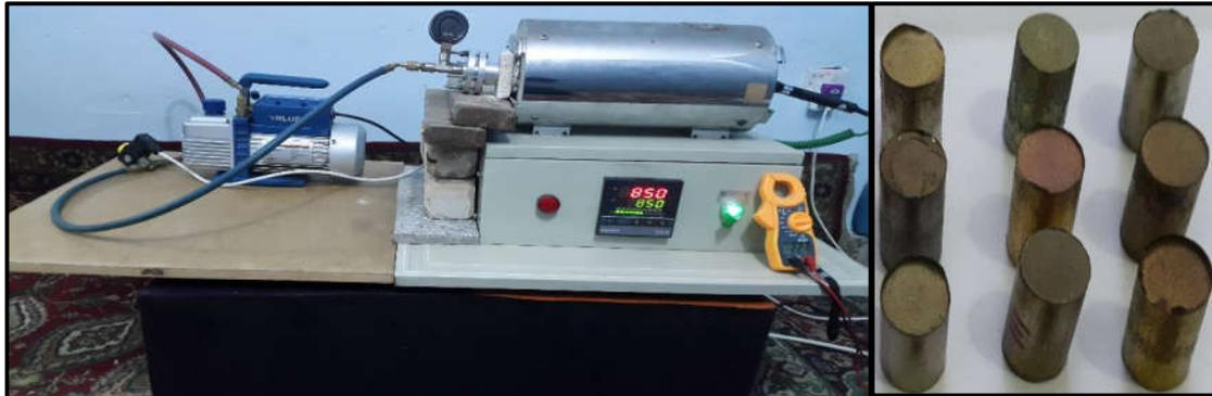
**Fig.5** Electrical furnace with a vacuum system & sintered samples
