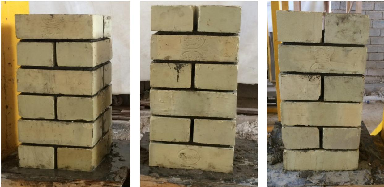
Figure 1: Set of three prisms constructed for test
