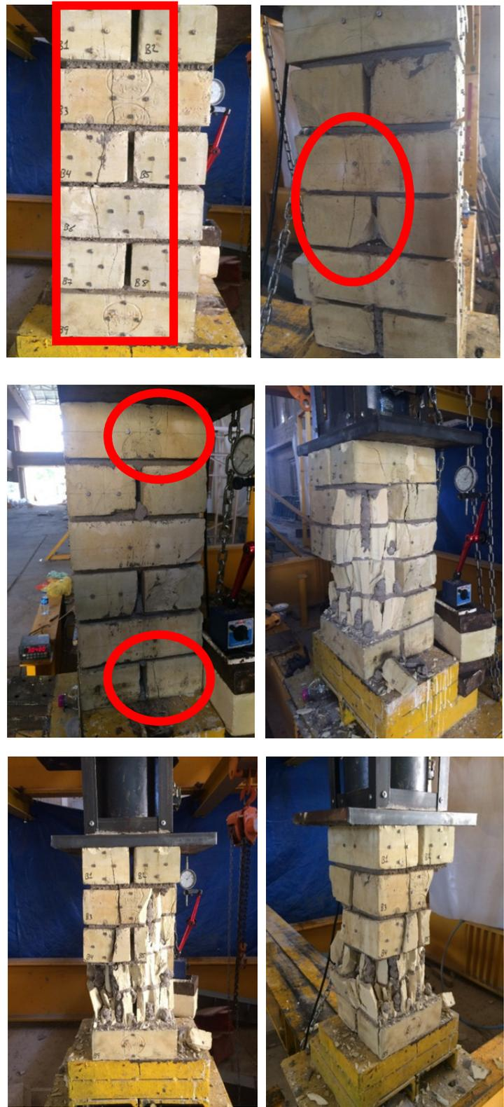
**Figure 8:** Cracks formation and failure of the clay masonry prisms
