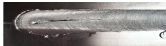
Figure 4: Specimen no.13 lack of filling defect.
