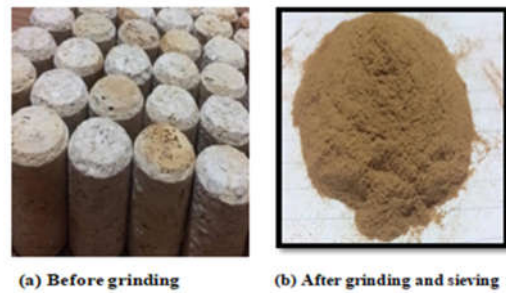
Figure 1: A sample of natural and grinded cork stopper particles.
