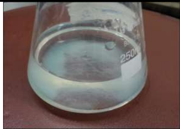
Fig 4. Precipitation of \text{Cr}^{+3} at pH 6.
