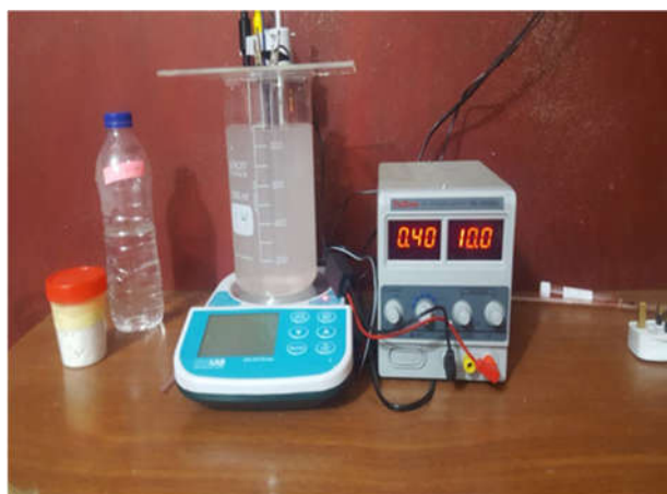
Figure 2: plate picture of EC cell in mid of experiment at Env. Eng. Labs
