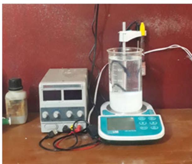
Figure 3: photographic picture of EC cell in end of experiment at Env. Eng. Labs
