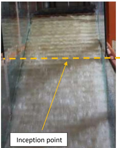
Figure 3: Inception point location for  $S_1$  model with discharge of  $0.0323 \text{ m}^3/\text{s}$
