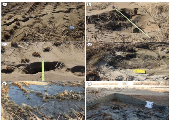
Figure 3: Field evidence of liquefaction occurred during the Pohang earthquake (a) linear chain of sand boils observed around the epicentral area, (b,d) isolated sand boils of larger than 1m in diameter observed in a rice farm and dry river bed ejecting fine sand/silty sand and coarse sand, (c) field photos showing isolated/ lenticular sand boil craters, (e) waterlogging in the rice farms immediately after an earthquake, (f) section of the sand boils where the soil samples were taken for grain size analysis [56]
