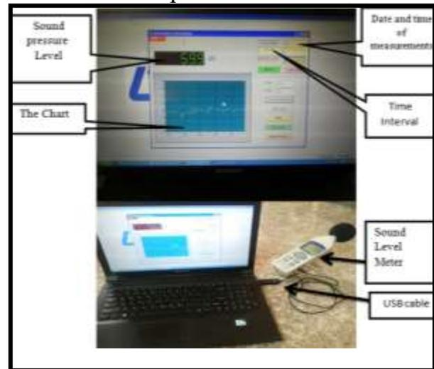
**Fig 2. Sound Level Meter connected to Laptop by Lutron program**
