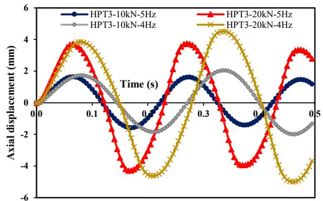
**Figure 15:** Variation of displacement with time of screw pile HPT3 subjected to seismic loading of intensities (10 and 20 kN) and frequency of 4 Hz and 5 Hz.
