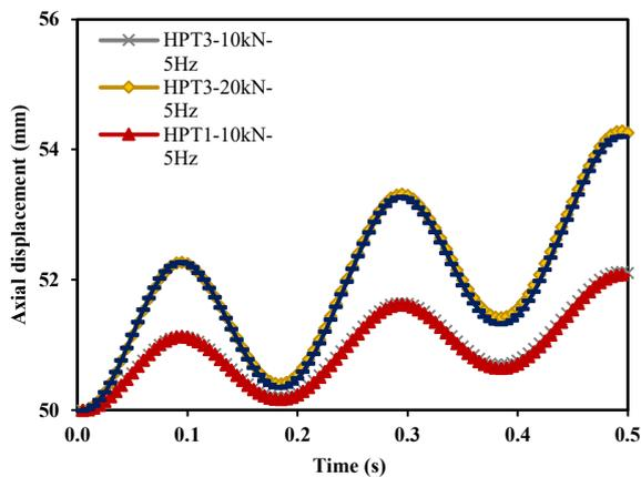
**Figure 14:** Axial displacement result of seismic loading (0.47g) and axial pullout loading (162 kN).
