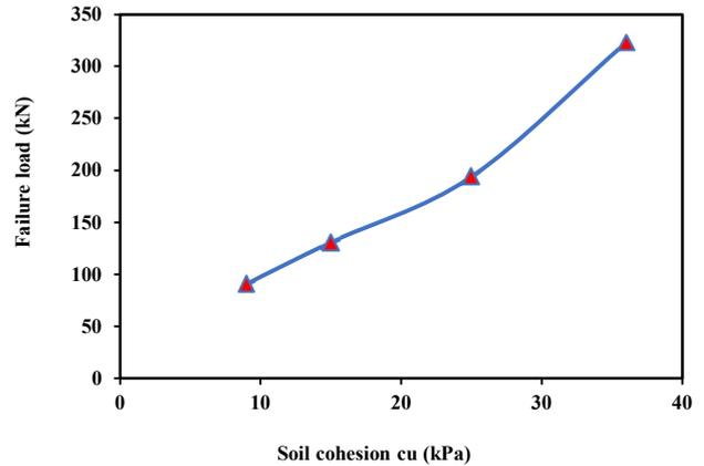
**Figure 11:** Relationship between failure pullout load of screw pile HPT and soil cohesion.
