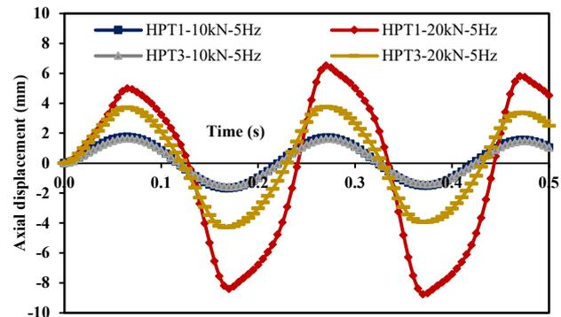
**Figure 16:** Effect number of helix-plate on axial displacement during seismic axial loading frequency of 5 Hz.
