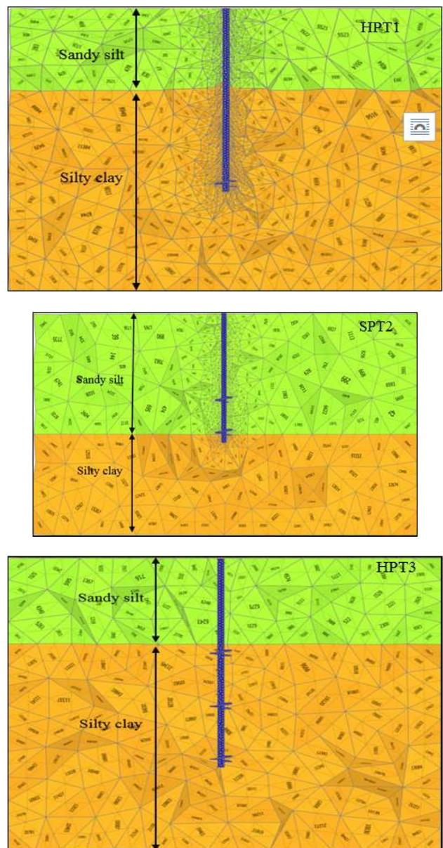
**Figure 8:** Typical mesh for screw piles HPT1, HPT2, and HPT3 analyzed in this study.
