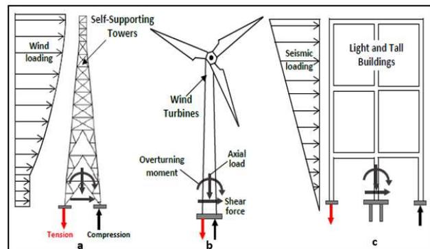
**Figure 1:** Uplift in (a) A transmission tower that has been subjected to wind loads, (b) A wind turbine is subjected to a load of wind, (c) Seismic loading on a residential structure [10].
