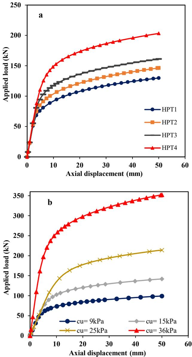
**Figure 10:** Variation of pullout load versus axial displacement of screw piles: a) screw piles inserted into two layers of soils, b) HPT3 inserted in one layer of soil having different cohesion
