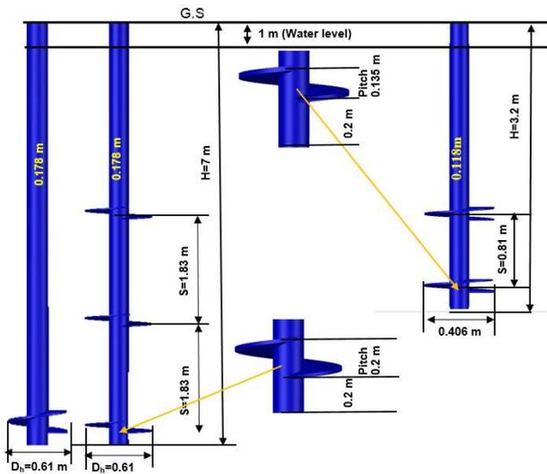
**Figure 3:** Geometry and dimensions of two screw piles used in the analysis.
