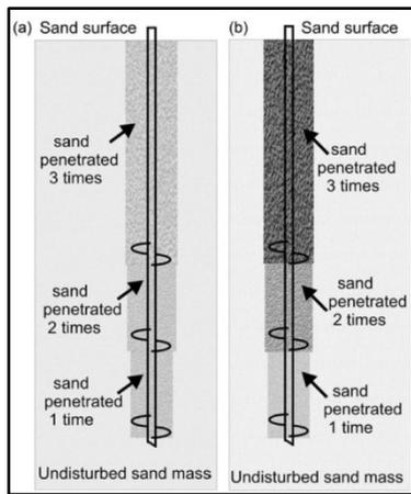
**Figure 6:** Illustration of the hypothesis for sand disturbance after installation of a three-helix pile: a) loose sand; b) dense sand[25].
