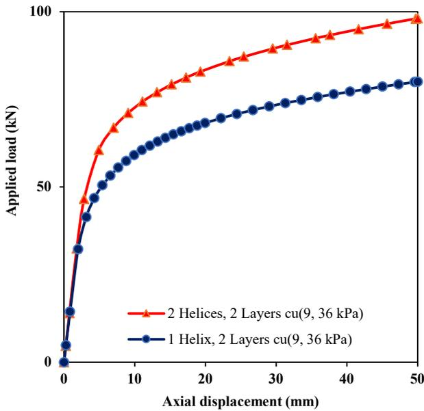
**Figure 13:** Variation of pullout load and axial displacement of screw piles (SPT1 and SPT2 inserted in two layers of soil).
