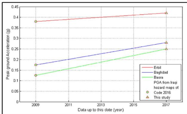
**Figure 9:** PGA values from the seismic design code of Iraq for version (2016) with that from study of [28].
