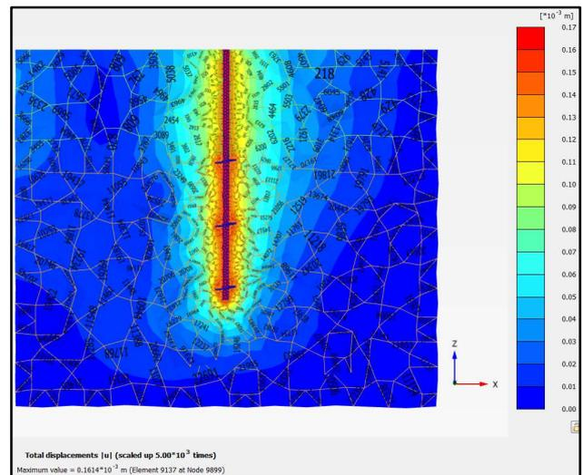
**Figure 12:** The displacement resulting from the self-weight of the screw pile.
