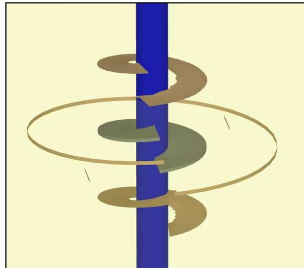
**Figure 5:** The soil-screw pile interface.
