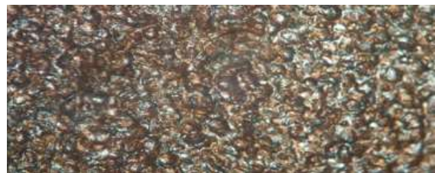
Fig. 5 optical microscopy with 200X after compacting at 650 Mpa
