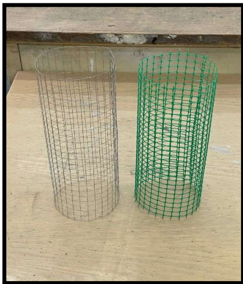
Figure 3: Cylindrical Steel and polymer reinforcement grids.
