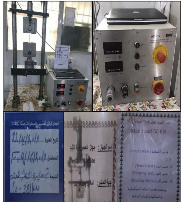
Figure 6: Tensile test instrument.
