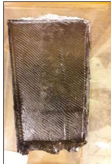
Figure 3: Carbon fiber with lamination resin.
