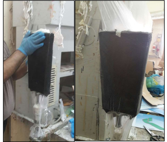
Figure 2: Carbon fiber layers.
