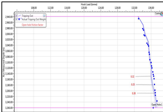
Figure 15: Friction Calibration during POOH of 8.25" BHA of Well-AG.
