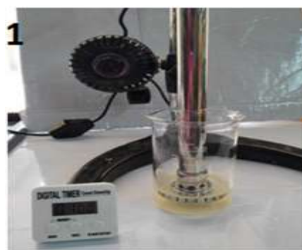
Fig. 4. Experiment procedure steps (1) adding membrane phase to internal phase
