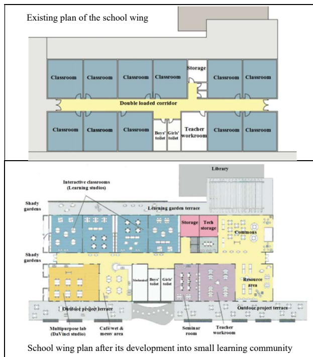
Figure 7: Hillel Academy of Tampa school primary grades wing plan before and after renovation [23].
