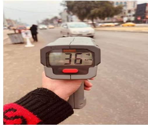
Figure 2: Speed Gun, Bushnell Velocity Speed Gun used for Speed Data Collection.
