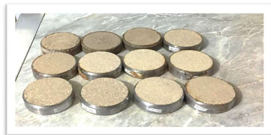
Figure 4: 12 specimens treated with 3,6,10% from (pp)
