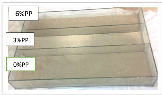
Figure 6 photo illustrates the compacted treated and untreated gypsum soil
