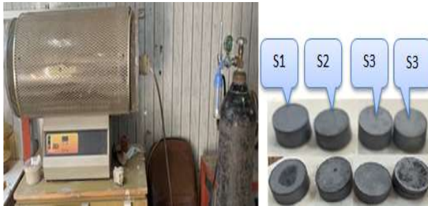
Figure 2: (a) Electrical furnace with an inert gas system, and (b) Samples after heat treatment
