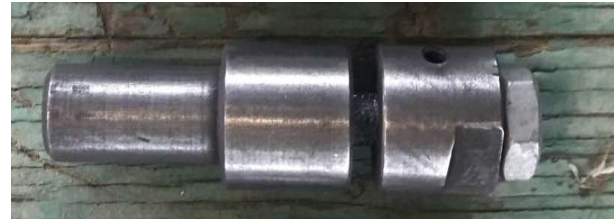
Figure 4: Bobbin tool with threaded tool
