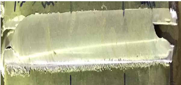
Figure 7, a: The upper side used threaded tool pin
