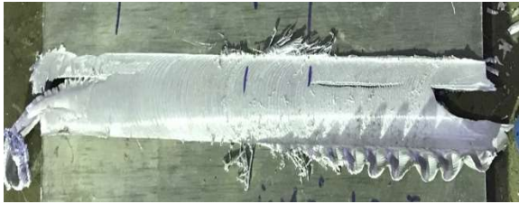
Figure 6, a: the upper side used cylindrical tool pin
