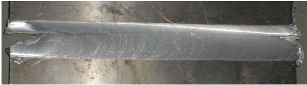
Figure 10, b: The lower side welded by tool threaded with two flat faces.
