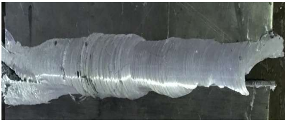
Figure 6, b: the lower side used cylindrical tool pin
