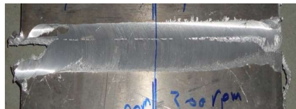
Figure 8, b: The lower side welded by square tool pin
