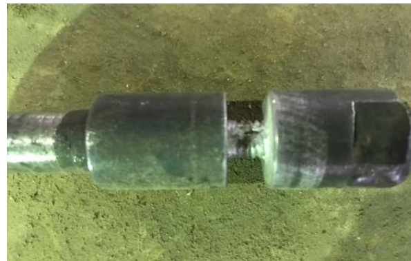
Figure 2, a: Threaded cylindrical with 2 flat surfaces
