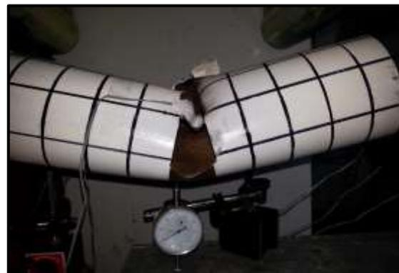
**Fig 5. Structural failure of the specimen BT4.**
