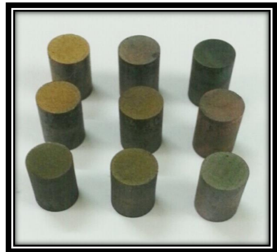
Fig 3: Samples after sintering (after different sintering temperature )
